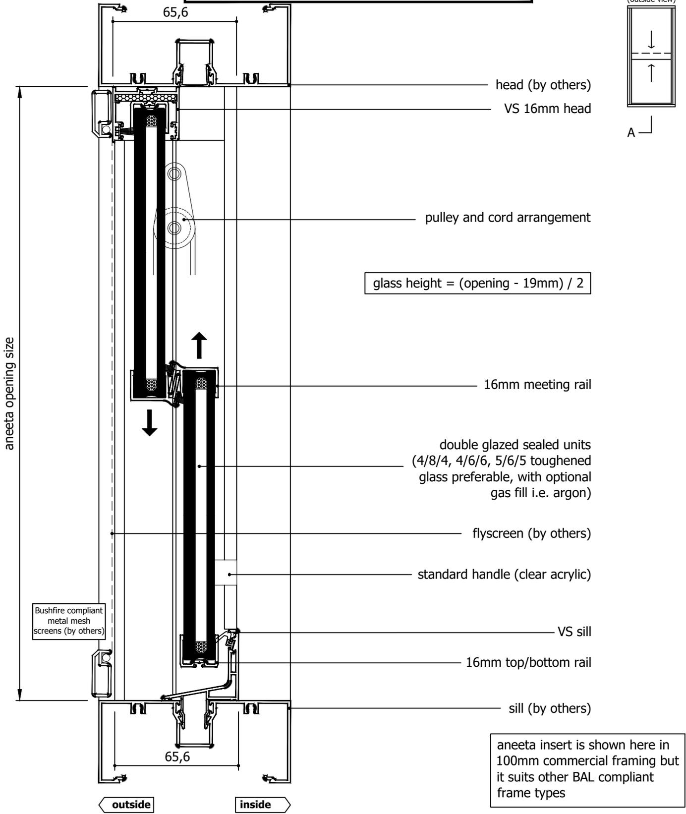
$$\text{glass height} = (\text{opening} - 19\text{mm}) / 2$$
