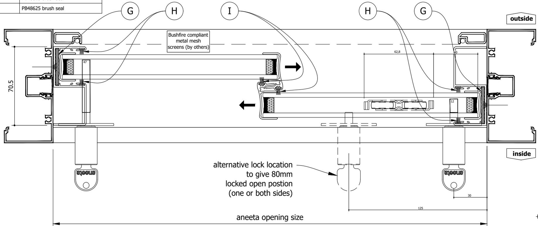
N:\Documentation\Website Downloads\4. Special Applications\2. Bushfire\HSF 2P22 SS A (B) - BAL12.5 to 40 2 pane 22mm DOUBLE GLAZED sashless horizontal sliders in aluminium frames SS.dwg
